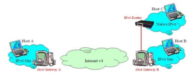
The 6to4 Gateway B that is a relay router is set as default route for 6to4 Gateway A. We will not announce our IPv6 Native Prefix using a routing protocol such as BGP4+. A native IPv6 prefix is assigned to the IPv6 router.
